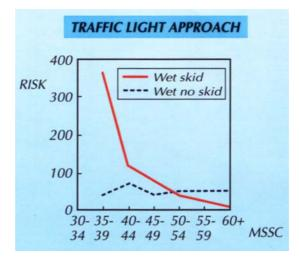
Arising out of this work, the "Skidding Standard" (HD 28/94) was implemented nationwide for Motorways and Trunk Roads in January 1988. It formalised the relationship between aggregate properties (including PSV), traffic levels and SFC and established levels of inservice skidding resistance that ensured a uniform risk of a wet skidding accident occurring over the whole network.
