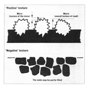
The classic associations between aggregate properties and texture depth have all been established from measurements on a range of surfacing types with one common feature, namely, "positive" texture depth.
