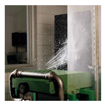
Figure 3.18 Composite picture showing The difference in the level of spray generated in the laboratory between a conventional smooth spray flap material (right) and spray suppressing media (left) (clear pass) Spray suppression devices
