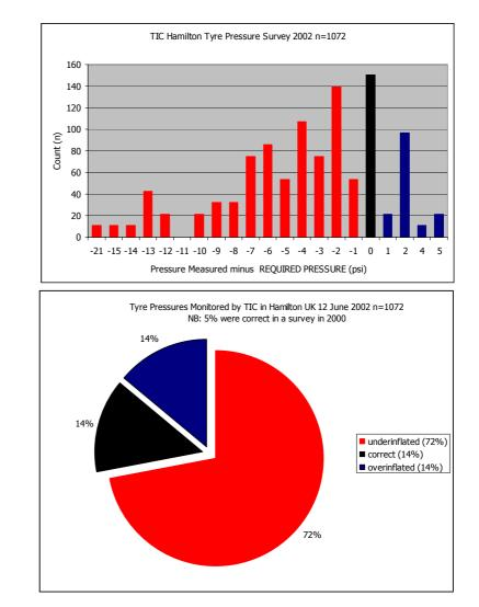
It must be said that the removal of tyre valve caps and the struggle with garage airlines is not a task many relish, but if both the cost implications of the reduced service life of the tyres and the effect of under inflation on handling were more widely publicised, more attention might be paid to maintaining tyres at the correct pressure.
