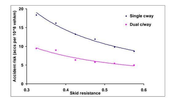
Figure 3.6b Relationship between overall accident risk and skid resistance for different types of site
