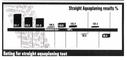
The automotive press carry out tests to give a limited perspective on the relative levels of performance expected, these tests usually compare the top 10 tyre brands. Common practice is to use one
