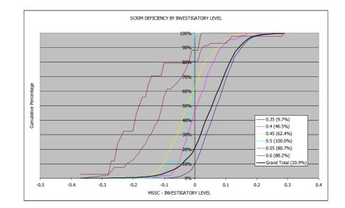
As can be seen from Figure 3.9 (representative of the data collected from 15 authorities), the single NRMCS statistic of approximately 20 per cent for one Authority is an oversimplified combination of many individual results with 10, 20, 40, 80 and even 100 per cent of MSSCs at or below the relevant investigatory levels.
