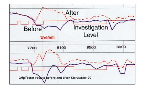
If the study by Hertfordshire of the effect of retexturing on wet-skid accident reduction (see Figure 3.15) can be reproduced elsewhere, and augmented to include the micro- and macro- texture state of the sections during the before and after periods, the true effect and whole life cost of these low cost retexturing processes may be better understood.
