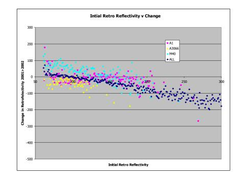
Figure 3.20 Change in retroreflectivity (2001 to 2002) versus initial retroreflectivity for 2001: RSMA ECODYN SURVEY
