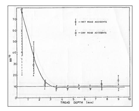
In the earlier work, the possible contributory effects of the behaviour of drivers who operate with low tread depth tyres were recognized. The reports recommendation of a 4/32 inch (3.2 mm) legal minimum tread depth was based upon assigning only 50 per cent of the projected accident reduction as a benefit. The remaining 50 per cent was not expected to materialize based upon the unchanged behaviour of the driver. However, the fifty-fifty split was subjective and was challenged.
