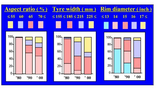
Isomura (2002) summarised how the aspect ratio, tyre width and rim diameter has changed for Toyota cars over the last 20 years, this shown in Figure 2.12.
