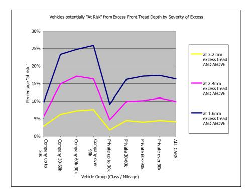
As part of this project, the TIC database was examined for evidence of tread depth imbalance. The findings, shown in Figure 2.20, suggest that approximately 4 per cent to 17 per cent of the cars surveyed are potentially "at risk" by virtue of the lesser tread depth on the rear tyres compared to that on the front tyres.
