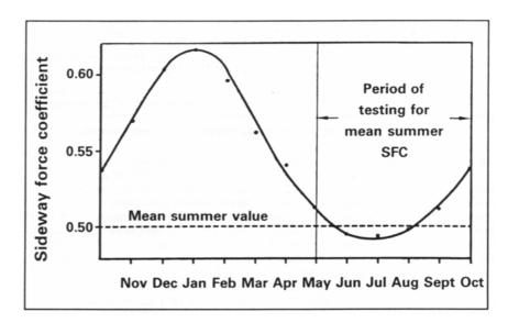
In the UK, there is a significant seasonal variation in skidding resistance, (as shown in Figure 3.2) with minimum values occurring during summer and early autumn. During the summer, dry polishing of the road's micro-texture occurs due to the action of traffic, and skid resistance values fall. Later in the year, when the road is wet for prolonged periods, wet polishing with gritty materials tends to restore the micro-texture and skid-resistance values rise.
