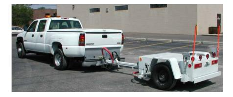
Evidence, particularly from The Netherlands, suggests that the monitoring of porous asphalt (the longest established "negatively textured" material) using locked-wheel dry-skid testing may be required to provide the engineer with a guide as to when signs warning of extended dry stopping distances on new construction should be removed (Jutteo and Siskens (1997)).
