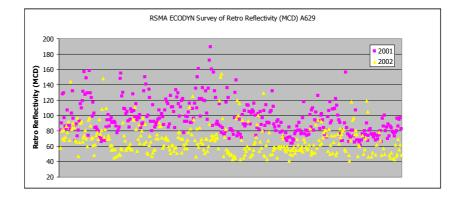
What must be observed is the potential for the retro-reflectivity to drop from an initial maximum high as the beads applied to the surface are lost, then to increase to a longer term equilibrium established shortly afterwards (with the onset of the exposure of new glass beads within the mass of the line as it slowly wears away).
