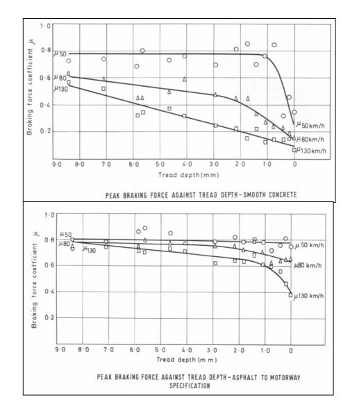
Published TRL work (Staughton and Williams (1970)) indicated a sudden loss in tyre traction below 1 mm tread (As shown in Figures 2.13 and 2.14), this knowledge combined with a need to prevent exposure of tyre steel bracing (that could lead to corrosion and explosive tyre failure), led to the introduction of a 1 mm minimum tread depth requirement.
