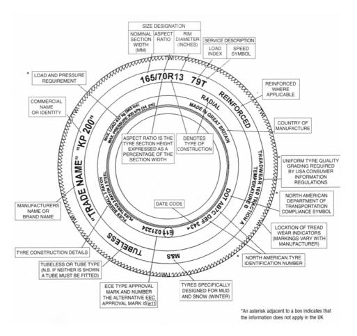
All tyres are designed to operate within a range of speed, load and temperature, the coding found on the side of the tyre provides the necessary detail. However, the correct tyre pressures for the vehicle are not marked on the sidewall.
