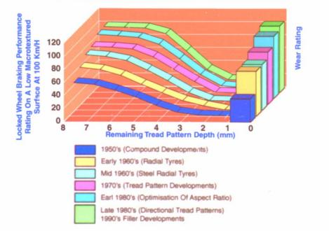
Figure 2.2 illustrates the almost three-fold increase in the wear resistance of a typical tyre between the mid 1950s and the 1980s, and the way in which the level of wet road holding has been improved as the tyre wears.
