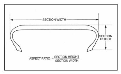
There are many fundamental properties of any tyre that can be changed by the technologist using the facilities of factory and test track, for example, aspect ratio as illustrated in Figure 2.11. However, the motorist may choose tyres of a different aspect ratio from standard fitment.
