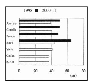
Figure 2.1 illustrates how the stopping distances for some Toyota vehicles (as an example) have reduced in just 2 years. The improved performance of tyres has contributed significantly to these benefits.
