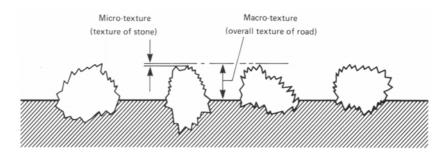
Micro-texture is the property of the individual aggregate particle, which, when combined with the free draining properties provided by the macro-texture in the wet, results in the effective skid resistance of the surfacing:
