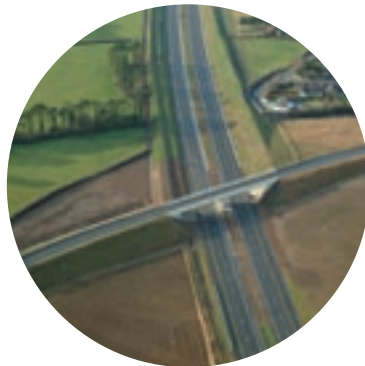
Separating opposing flows and using split-level junctions reduce opportunities for conflict
