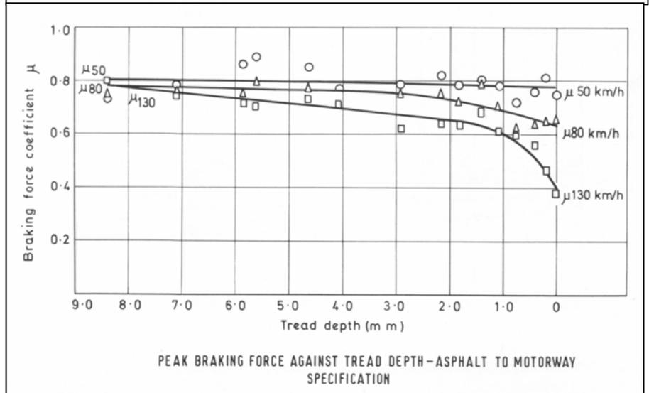
Published TRL work (Staughton and Williams (1970)) indicated a sudden loss in tyre traction below 1 mm tread (As shown in Figures 2.13 and 2.14), this knowledge combined with a need to prevent exposure of tyre steel bracing (that could lead to corrosion and explosive tyre failure), led to the introduction of a 1 mm minimum tread depth requirement.
