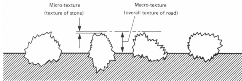
Micro-texture is the property of the individual aggregate particle, which, when combined with the free draining properties provided by the macro-texture in the wet, results in the effective skid resistance of the surfacing:
