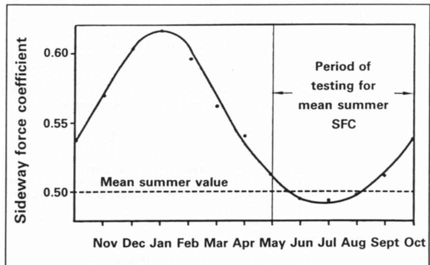
In the UK, there is a significant seasonal variation in skidding resistance, (as shown in Figure 3.2) with minimum values occurring during summer and early autumn. During the summer, dry polishing of the road's micro-texture occurs due to the action of traffic, and skid resistance values fall. Later in the year, when the road is wet for prolonged periods, wet polishing with gritty materials tends to restore the micro-texture and skid-resistance values rise.
