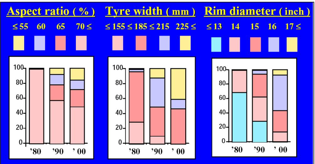
Isomura (2002) summarised how the aspect ratio, tyre width and rim diameter has changed for Toyota cars over the last 20 years, this shown in Figure 2.12.
