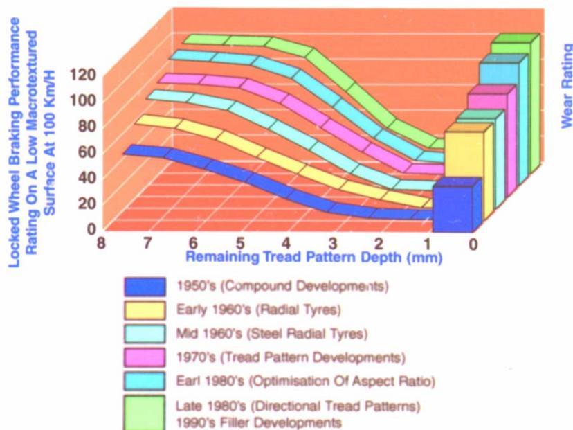
Figure 2.2 illustrates the almost three-fold increase in the wear resistance of a typical tyre between the mid 1950s and the 1980s, and the way in which the level of wet road holding has been improved as the tyre wears.
