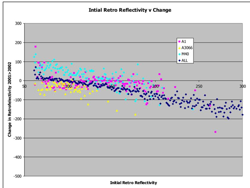
This plot appears to identify where lines have been replaced (new lining shows as an increase in retro-reflectivity between 2001 and 2002) This indicates replacement is generally taking place when retro-reflectivity is well below the proposed Highway Agency investigatory level of 100mCd and the minimum level suggested by the industry.
