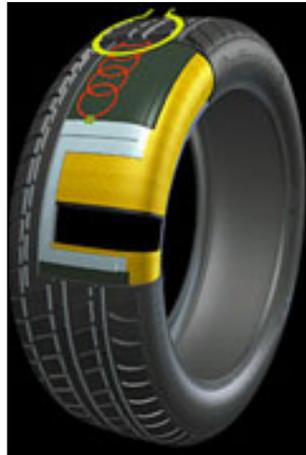
The “smart tyre” concept is one in which the performance of existing tyres can be optimised by integrating their characteristics into an adaptive suspension/braking/chassis system, measuring the deformations of the tyre profile and tread contact area and using this information to optimise the characteristics of the other systems.
