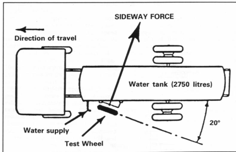
The HGV-based SCRIM (Sideway force Co-efficient Routine Investigation Machine, illustrated in Figure 3.4) is presently the main device used for measuring the skid-resistance of complete networks.
