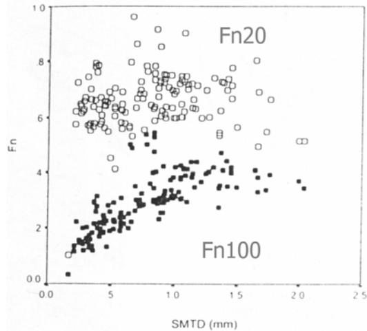
The Skidding Standard is geared around wet-skid-resistance measurements taken at relatively low speed. However, the level of wet skid resistance delivered at high speeds will depend to a great extent on the surface texture.
