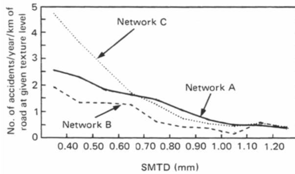
This research linking texture depth to accident risk supports the use of the 1.5mm minimum texture depth requirement for new construction of high speed roads in the UK.
