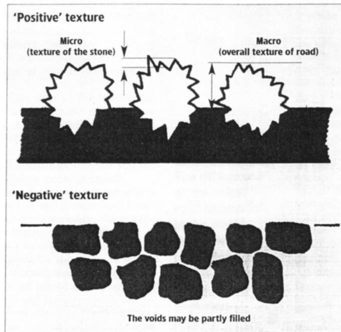
The classic associations between aggregate properties and texture depth have all been established from measurements on a range of surfacing types with one common feature, namely, "positive" texture depth.
