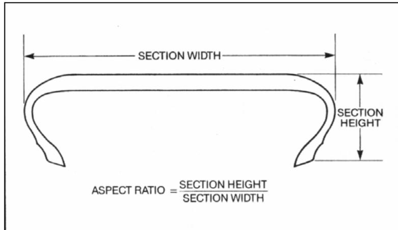
There are many fundamental properties of any tyre that can be changed by the technologist using the facilities of factory and test track, for example, aspect ratio as illustrated in Figure 2.11. However, the motorist may choose tyres of a different aspect ratio from standard fitment.
